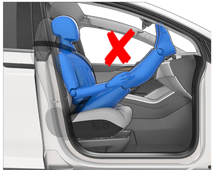
Incorrect seating position - the passenger must not slide forward on the seat cushion:
