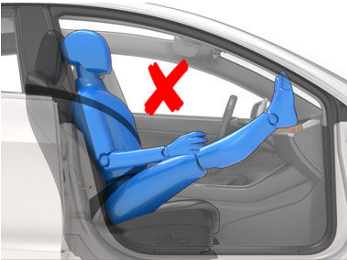
Incorrect seating position - the passenger must not slide forward on the seat cushion:
