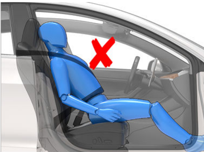
Incorrect seating position - the passenger must not recline the backrest to a laying down position when the vehicle is moving:
